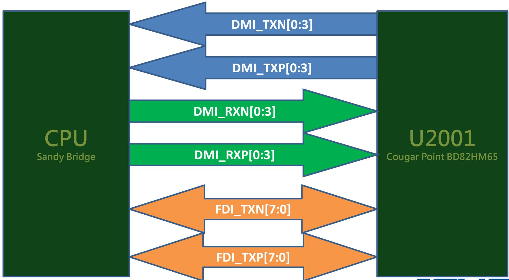
➤ Connection problems between CPU, PCH, RAM and GPU
