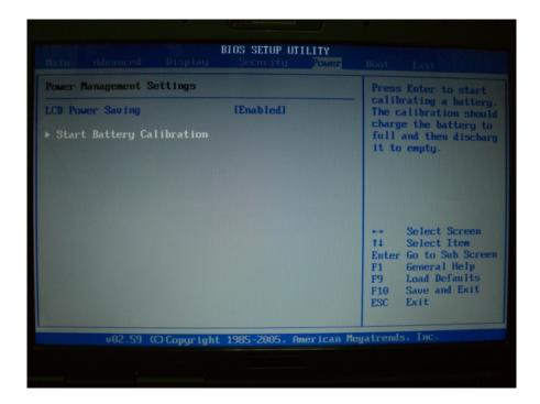
After long time incomplete charge/discharge cycles, the battery meter becomes less and less accurate (the total power capacity is not significantly affected, however). Battery gauge needs to "learn", this item helps users to recalibrate the battery gauge. In the learning process, users need to follow system BIOS instruction to Insert/remove the AC adapter so that a complete reset and learning cycle may start.
